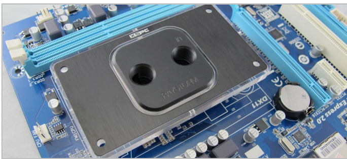
5. Place the waterblock onto the CPU and line-up the mounting plate with the holes on the motherboard.
