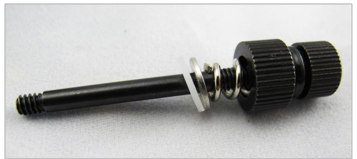
6. Place a spring and washers over each bolt. Bolt >Nut >Spring >Metal washer >Plastic Washer
