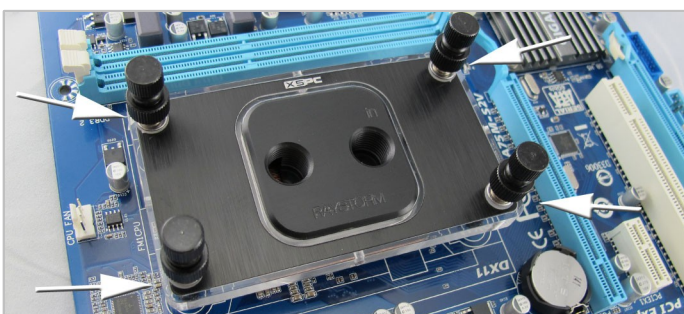
7. Place each of the bolts through the mounting plate and loosely screw into the backplate using the knurled section of the bolt [A]. When all 4 bolts are loosely fitted, tighten each bolt [A].
