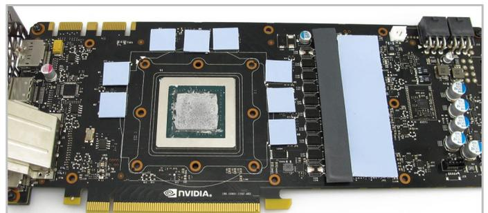
11. Remove the tape from both sides of the thermal pads. Place the blue and grey pads on the ten positions shown above and finally apply thermal paste to the GPU core.
