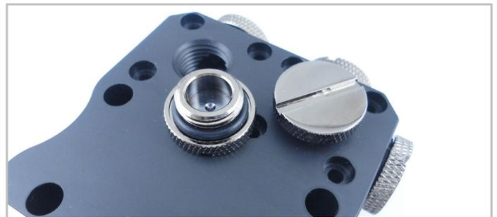
2. Use the G1/4" blanking plugs to block the unused ports.
