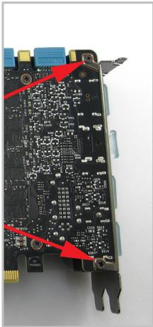
10. Use two of the provided screws and two nuts to secure the bracket. This must be done before the block is fitted.
