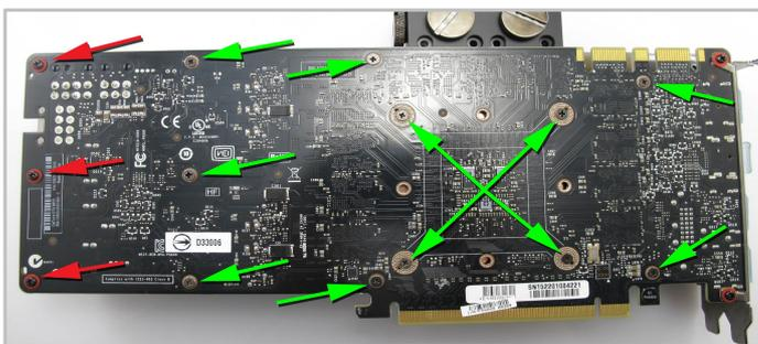
12. Now fit the original small screws to the positions marked above in green and the supplied screws and washers in positions marked red. You should gradually tighten each screw to apply even pressure..
