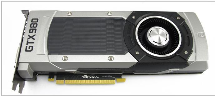
6. Before handling the card you should take precautions to avoid static damage. Remove the GTX 980 card from the box ready for installation.
