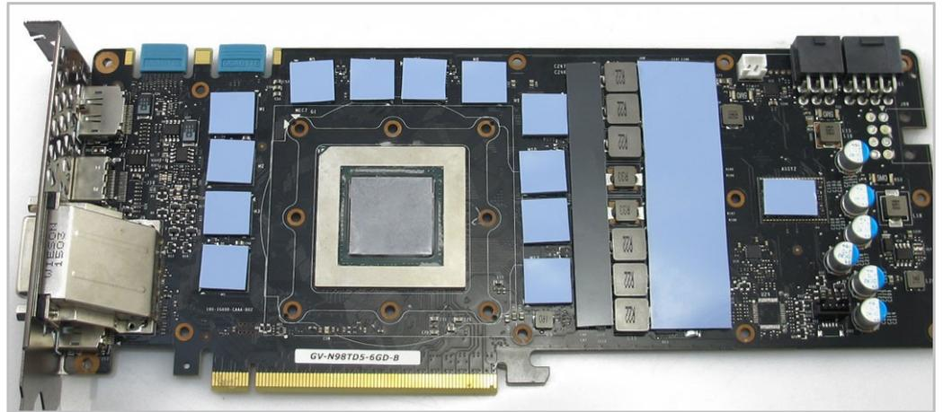
11. Remove the tape from both sides of the thermal pads. Place the blue and grey pads on the fifteen positions shown above and finally apply thermal paste to the GPU core. Place the waterblock on the card to line up the screw holes and then flip it over (make sure the thermal pads stay in place).
