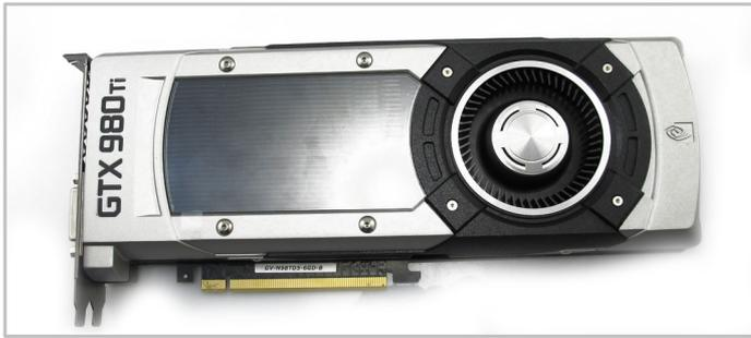
6. Before handling the card you should take precautions to avoid static damage. Remove the GTX 980 Ti card from the box ready for installation.
