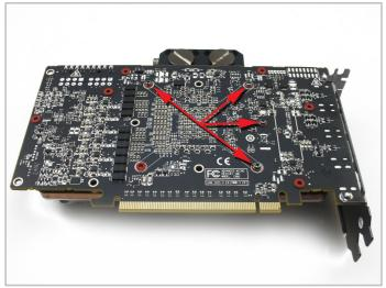
**3**. Fit the original screws to the positions marked above. Do not over tighten the screws as this may bend the card and cause permanent damage.
