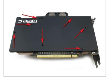
**4**. Place the backplate on the back of the card. Attach the backplate to the block using the provided screws.
