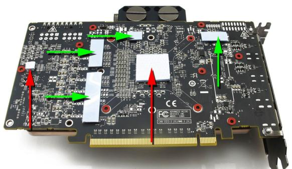
2. Flip the card over (make sure the front thermal pads stay in place). Place the red washers over the screw holes shown above. Now remove the protective film from both sides of the thermal pads. Place the 1.5mm pads in the positions marked in red and the 1mm pads in the positions marked in green.
