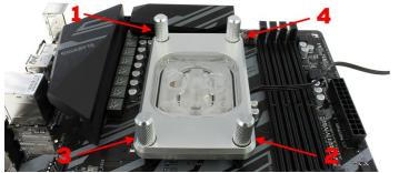
5. Place a nut onto each post and gradually tighten them. You should tighten each nut in stages. e.g. 1,2,3,4,1,2,3,4,1,2,3,4, until each nut is fully tightened.
