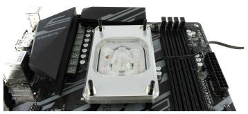
3. Place the waterblock over the posts and onto the CPU.
