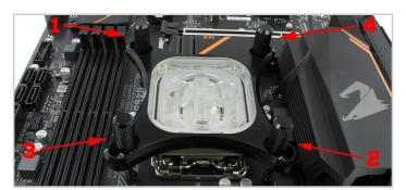
**5.** Place a nut onto each post and gradually tighten them. You should tighten each nut in stages. e.g. 1,2,3,4,1,2,3,4,1,2,3,4, until each nut is fully tightened.
