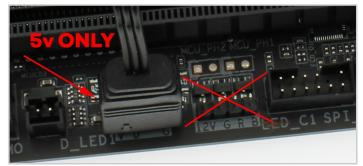
6. Connect the 5v 3pin aRGB plug to your motherboard RGB header or RGB controller.
