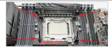
2. Screw the short end of the M4 post into each of the four holes around the socket.
