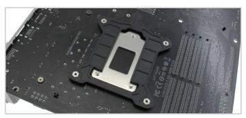
2. Make sure the 4 screw threads on the backplate line up with the holes on the motherboard. Apply pressure to secure the backplate.
