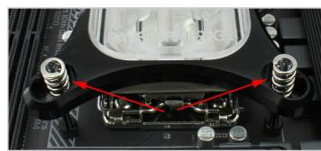
4. Place a spring over each of the four posts and into the wells on the hold down bracket.
