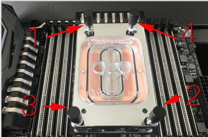
5. Place a nut onto each post and gradually tighten them. You should tighten each nut in stages. e.g. 1,2,3,4,1,2,3,4,1,2,3,4, until each nut is fully tightened.
