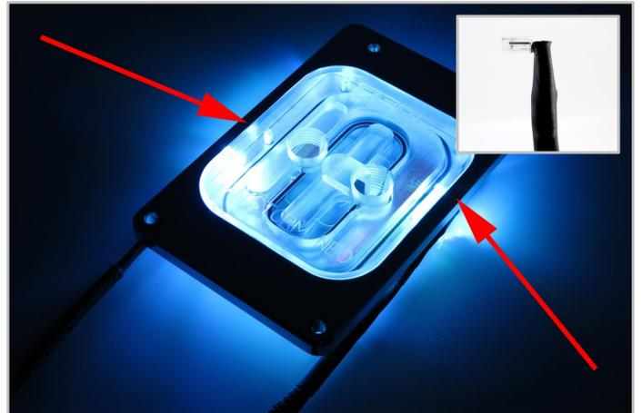
6. Push the LEDs into either side of the waterblock and connect them to the RGB controller. Use the needle connectors to connect the LEDs to the controller.
