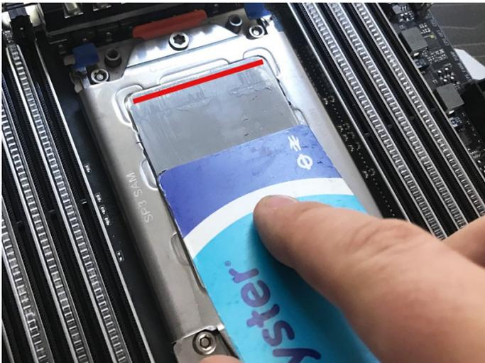
1. Apply a thin layer of thermal paste to the CPU's IHS. Start with a thin line at the top and spread out the paste evenly using a credit card.
