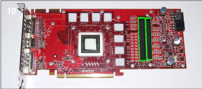
**10.** Remove the tape from both sides of the thermal pads and place them on the highlighted locations on the right of the card. Next apply thermal paste to the memory chips and the GPU core.
