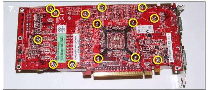
**7.** Turn the card on its back and remove the 14 screws highlighted above.
