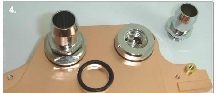
4. If you are using G1/4" barbs/fittings with a long thread you will need to use the supplied rings to avoid blocking the flow. Attach the barbs to your chosen ports using an adjustable spanner. Make sure the o-rings are fully compressed.
