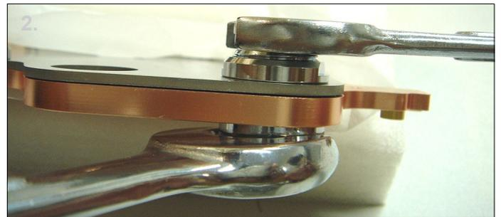
2. **IMPORTANT:** When you install the G1/4" fittings or plugs in steps 2,3 you will need a second wrench on the reverse side of the bulkhead fitting to make sure it doesn't unscrew.
