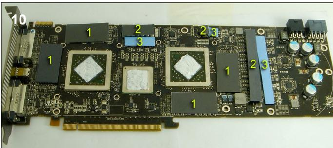
**10.** Remove the tape from both sides of the thermal pads. Place 4 black pads on the memory location marked 1 and place the other 3 black pads on the locations marked 2. Now place the thicker blue pads on the locations marked 3 it is important not to mix-up the blue and black pads. Next apply thermal paste to the chipset and the GPU cores.
