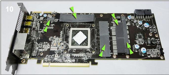
**10.** Remove the tape from both sides of the thermal pads and place the thermal pads in the five locations highlighted above. Now apply thermal paste to the GPU core.
