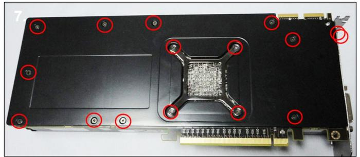
**7.** Remove the two screws on the bracket next to the DVI ports. Now turn the card on its back and remove the 14 screws highlighted above.
