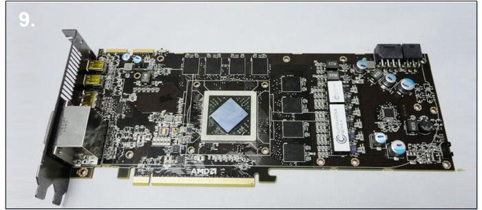
**9.** Clean the thermal paste from the GPU core ready for installation. Remove any residue left from the thermal pads.
