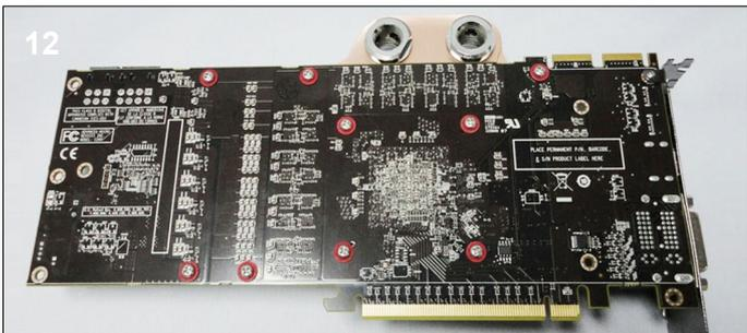
**12.** Finally use the 9 provided screws and washers to attach the waterblock to the card. It's best to start with the four screws around the GPU to apply the correct pressure to the core, followed by the five outer screws. Do not over tighten the screws as this may bend the card and cause permanent damage.
