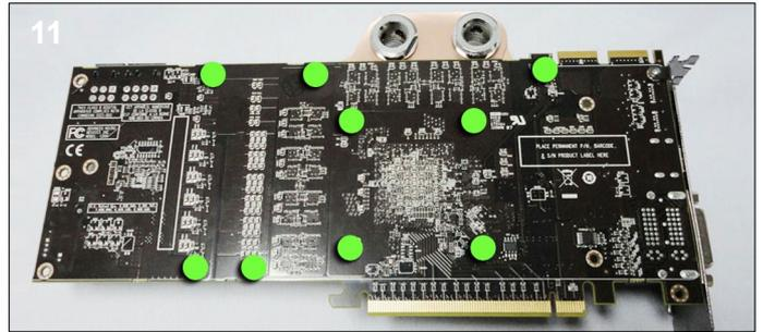
**11.** With the copper side of the waterblock facing up, place the card over the block and line up the screw holes. Make sure the thermal pads stay in place.
