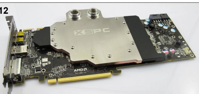
12. Do not over tighten the screws as this may bend the card and cause permanent damage. The card is now ready for use. When you first boot it is advisable to use ATItool or other software to check the core temperature. If the temperature is high you will need to remount the block.
