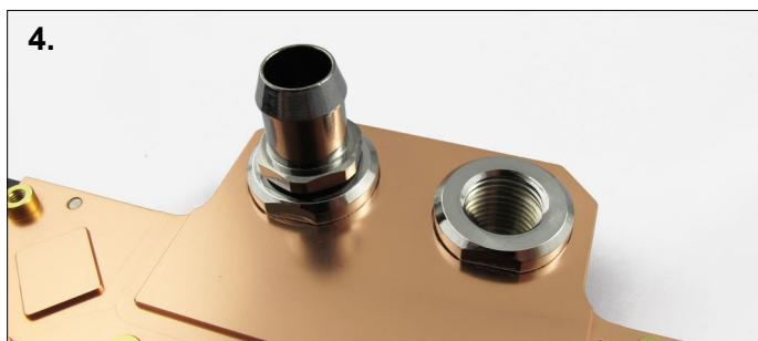
**4.** If you are using G1/4" barbs/fittings with a long thread you will need to use the supplied rings to avoid blocking the flow. Attach the barbs to your chosen ports using an adjustable spanner. Make sure the o-rings are compressed.
