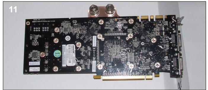
**11.** With the copper side of the waterblock facing up place the card over the block and line up the screw holes.
