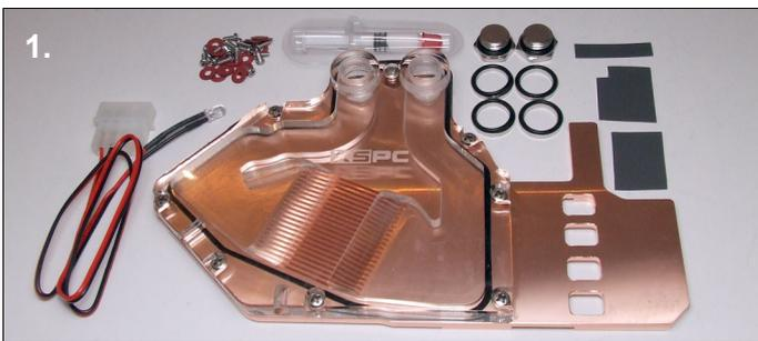
1. The waterblock is designed for SLI setups so you can fit the G1/4" fittings to either side of the block. Decide which configuration is best for your system.
