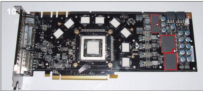
**10.** Remove the tape from both sides of the thermal pads and place them on the mosfets to the right of the card. Next apply thermal paste to the memory chips and the GPU core.
