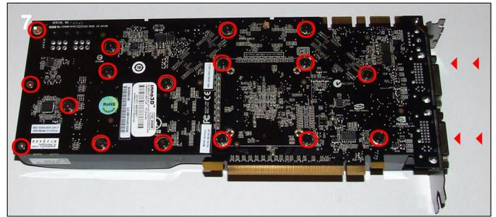
**7.** Remove the two screws next to the DVI ports then turn the card on its back and remove the 17 screws highlighted above.
