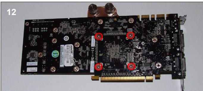
**12.** Finally use the 13 provided screws and washers to attach the waterblock to the card. It is best to start with the 4 screws around the GPU to apply the correct pressure to the core. Do not over tighten the screws as this may bend and damage the card.
