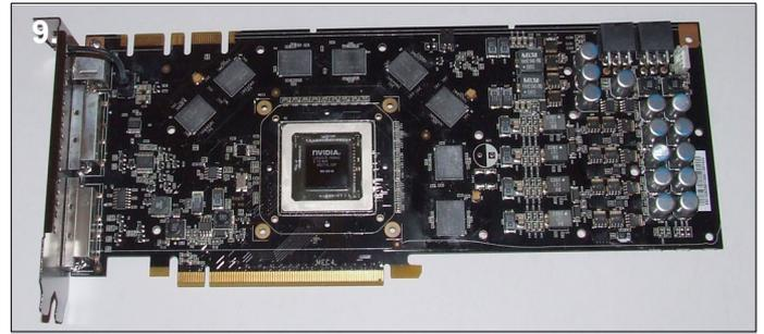
**9.** Clean the thermal paste from the GPU core ready for installation. Remove the old thermal pads and clean any residue..
