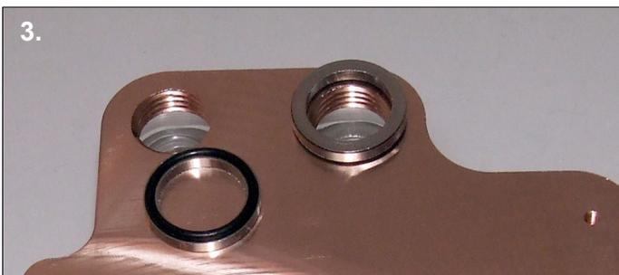
3. If you are using G1/4" barb/fittings with a long thread you will need to use the supplied rings to avoid blocking the flow.
