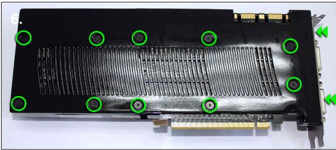
**6.** When handling the card you should take precautions to avoid static damage. Turn the card on its back and remove the 10 screws on the backplate highlighted above. Also remove the two screws near the DVI ports.
