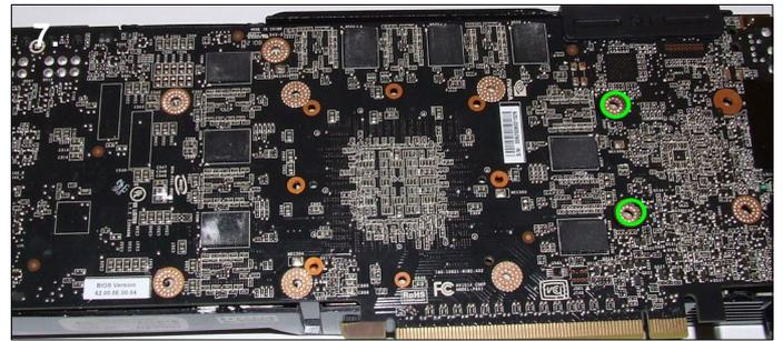
**7.** Carefully remove the nvidia backplate and unscrew the two screws highlighted above.
