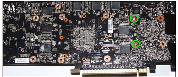
**11.** With the copper side of the waterblock facing up, place the card over the block and line up the screw holes. Make sure the thermal pads have stayed in place and lightly screw two screws with washers into the block through the holes highlighted above and replace the nvidia backplate.
