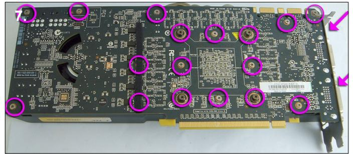
**7.** Remove the two screws on the bracket next to the DVI ports. Now turn the card on its back and remove the 17 screws highlighted above.
