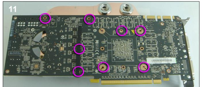
**11.** Place the waterblock on the card and then fill it over and line up the screw holes. Make sure the thermal pads stay in place. Now use 8 of the screws and washers to attach the waterblock to the card. Do not over tighten the screws as this may bend the card and cause permanent damage.
