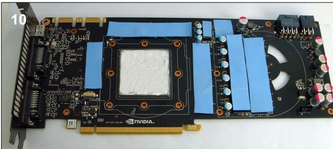
**10.** Remove the tape from both sides of the thermal pads and place them on the 7 locations shown above. Next apply thermal paste to the GPU core.
