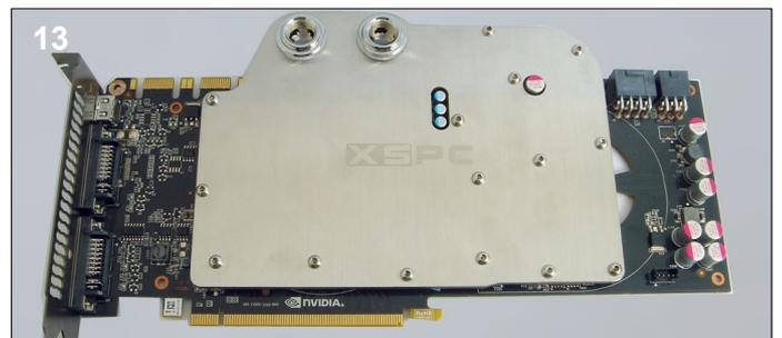
**13.** The card is now ready for use. When you first boot it is advisable to use ATItool or other software to check the core temperature. If the temperature is high you will need to remount the block.
