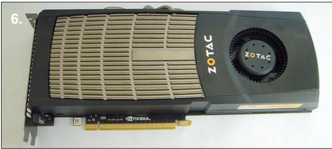
**6.** Before handing the card you should take precautions to avoid static damage. Remove the GTX480 card from the box ready for installation.
