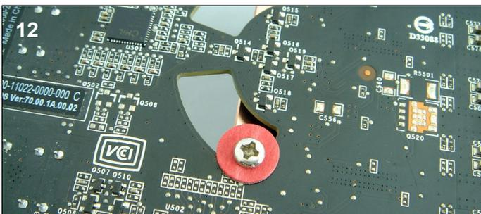
**12.** Finally use the large washer and last screw to attach the block through the cutout in the card.
